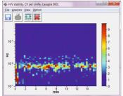
**VIBRATION ANALYSIS.** Sorting and spectral analysis of signal sections above thresholds, according to the European regulations on strong vibrations in structures. Automatic editable reports including tables and figures.
